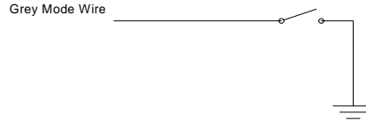
Figure 6: Mode Control Switch Wiring
